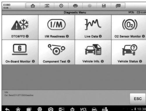
**Figure 4-14 Sample OBDII Diagnostic Menu**
