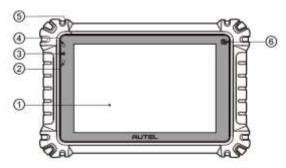
Figure 2-1 Tablet Front View
