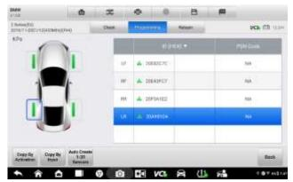
Figure 5-5 Sample Copy by Activation Function Main Screen
