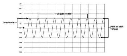
Figure 19-1 Sample Sinusoidal Waveform
