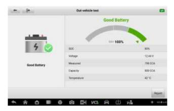
Figure 9-14 Sample Out-vehicle Test Result Screen
