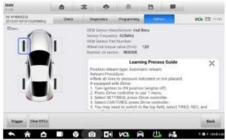
Figure 5-8 Sample Relearn Function Main Screen
