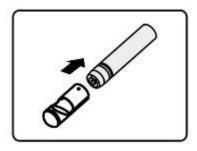
2. Slip the end of the accessory over the imager head and then fix the accessory.
