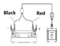
Figure 9-2 Connecting to a Battery
