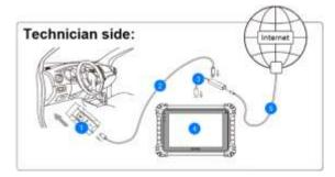
Figure 8-1 Sample connection diagram on Technician side
