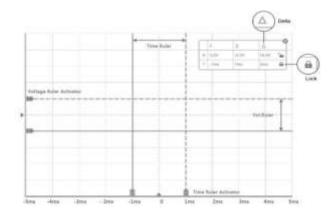
Figure 19-8 Measurement Rulers Display
